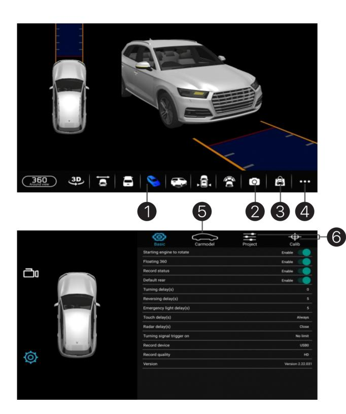
360 AVM Camera Settings: 360AVM function is optional, the device may not including Go to [Settings]--[Reverse mode]--[Reverse video input] --Select 360AVM pro to active 360AVM function Set up the camera Format to match Cameras for camera video display
